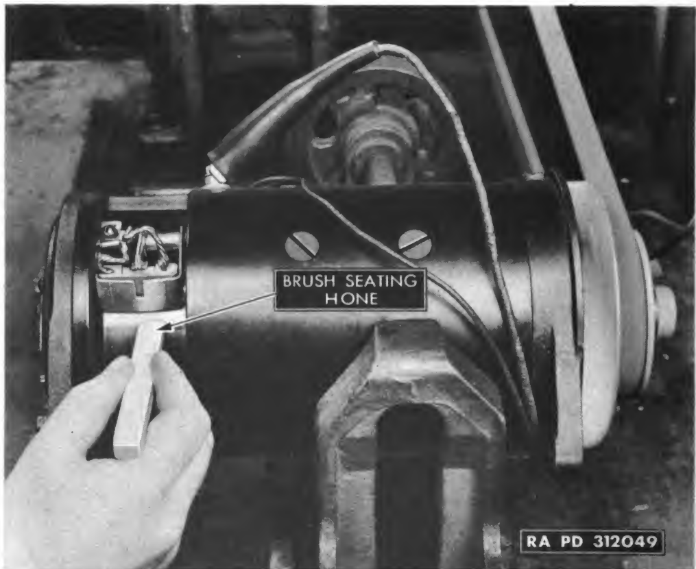
Figure 22—Using Brush Seating Hone (41-H-2387) to Seat Brushes
